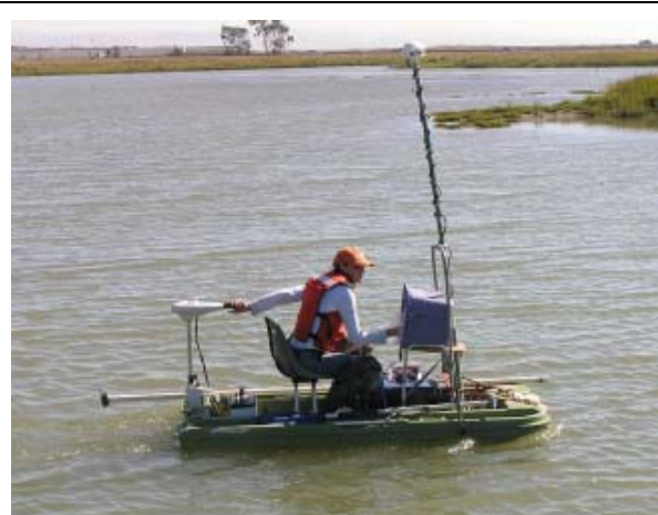
Figure 6. Bathymetry survey at Guadacanal
