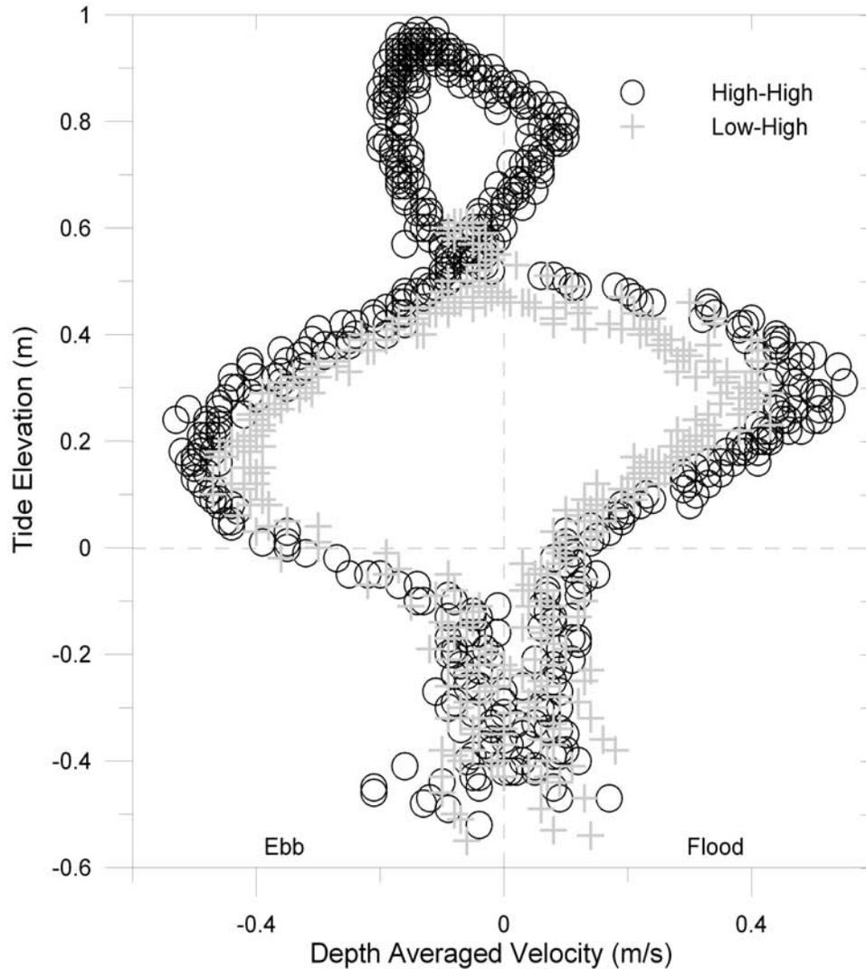
**Figure 6.** Velocity-stage height relationship from the profiler depth averaged velocity data in creek 6. The empty circle symbols represent all high-high conditions and the cross symbols represent all low-high tides. Note the “figure-8” shape and the three instances where the trends in the data cross the 0.0 m/s line, indicating flow reversals.
