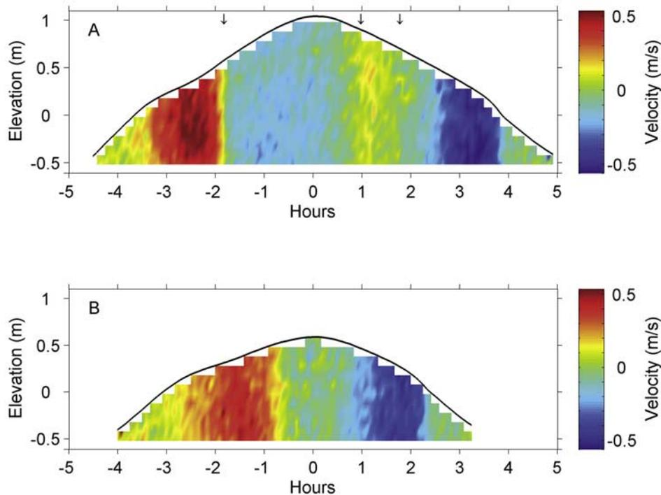
**Figure 5.** Time series of velocity profiles from creek 6 on June 5. Figure 5a corresponds to high-high tide and Figure 5b is for the low-high tide. Reds indicate upstream flow and the blues indicate downstream flow. Note the three sharp flow reversals that occur on the flood and ebb tide stages of the high-high tide, and the single reversal on the low-high tide. Arrows show flow reversals summarized in Table 1 and the black line is tide elevation.
