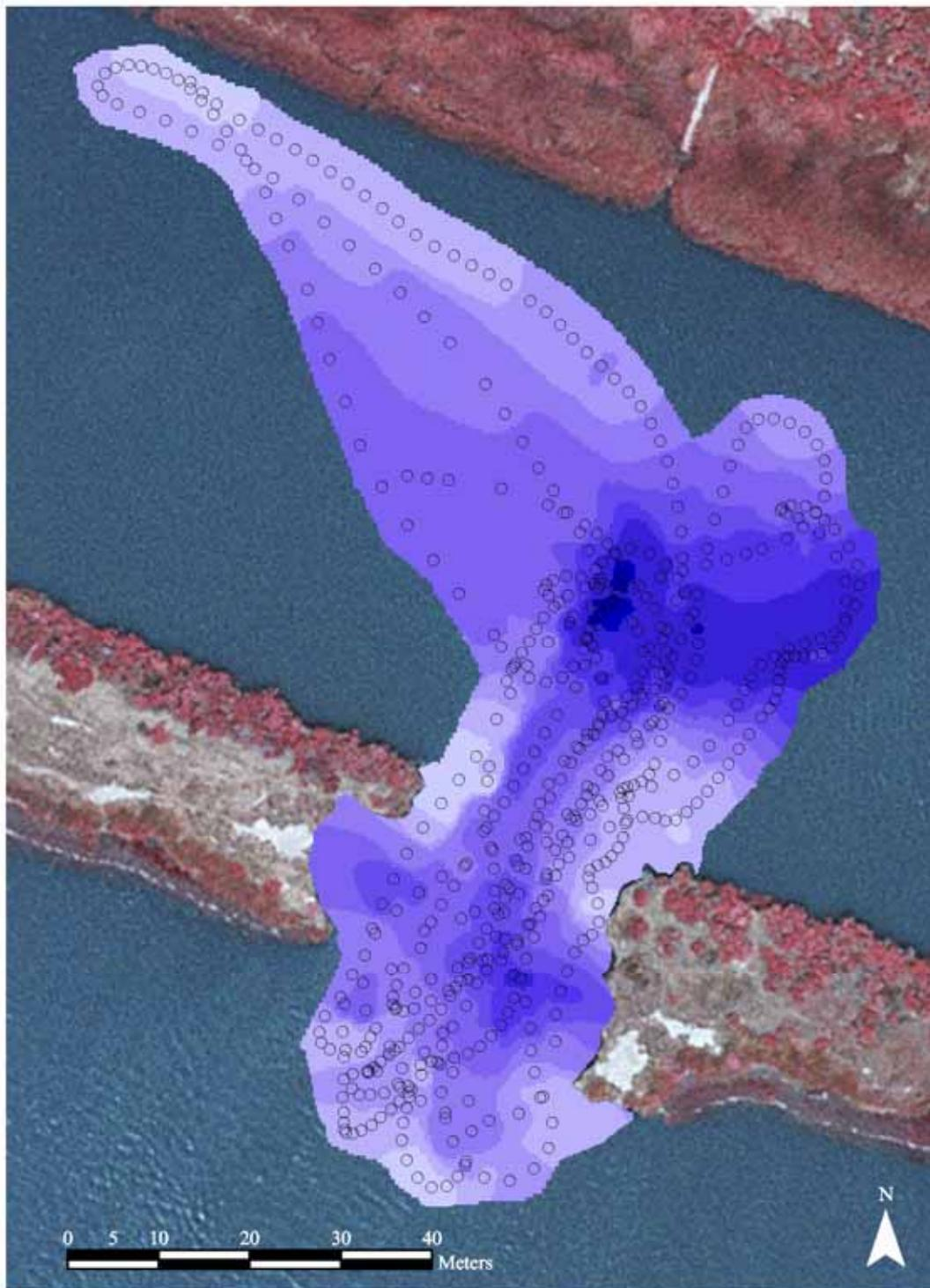
Figure 49. Relative bathymetry of South Slough and the Pond 3 breach, winter 2004-2005, Napa-Sonoma Marshes Wildlife Area, CA. Circles show data points; darker areas of bathymetric grid are deeper.
