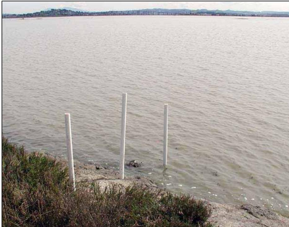
Figure 4. Location of erosion pins (indicated by yellow circles) installed at China Slough, Napa-Sonoma Marshes Wildlife Area, CA.
