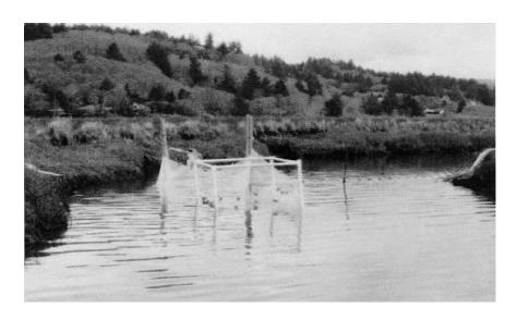
Figure 2. Modified fyke net deployed across a tidal channel in the reference marsh.
