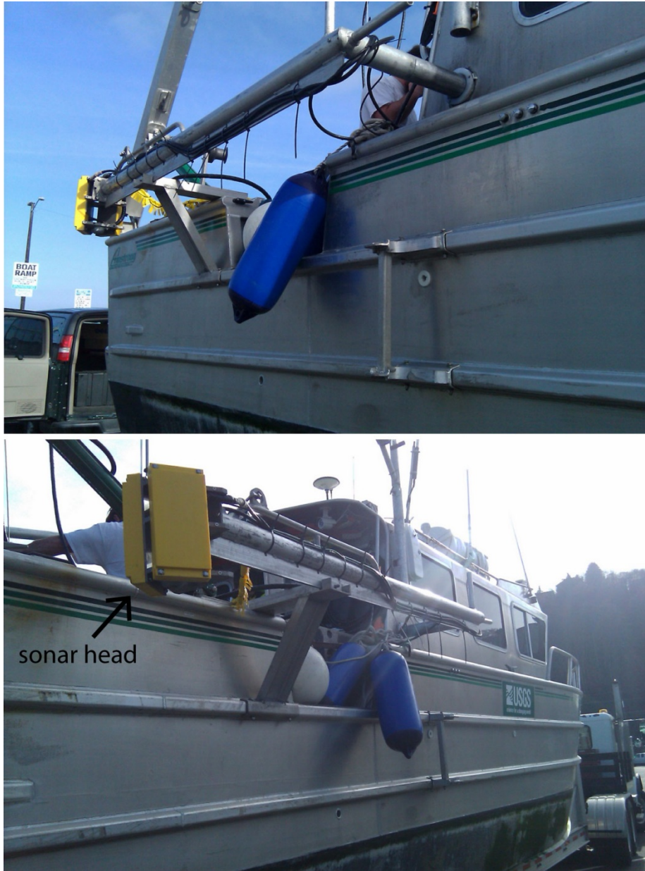
Figure 3. Fore and aft views of the SWATHplus sonar pole mount on the U.S. Geological Survey Coastal and Marine Geology R/V Parke Snively .
