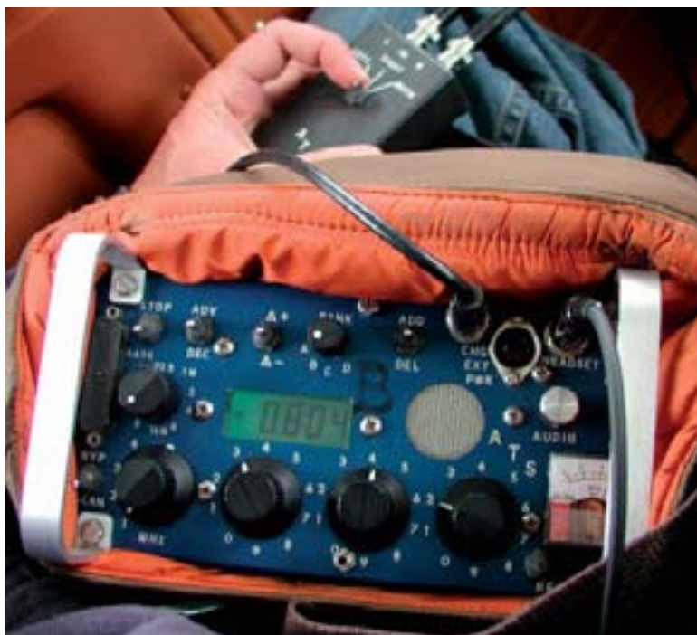
FIGURE 7.7 VHF receiver and switch box used for aerial tracking in conventional telemetry studies
