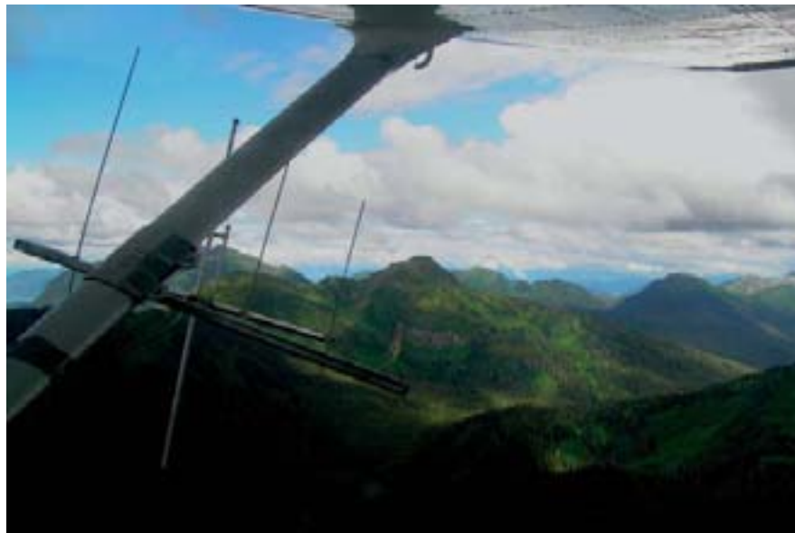
FIGURE 7.8 Four-element Yagi antenna mounted on aircraft strut
